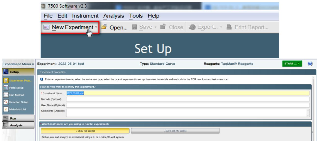
Select **7500 (96 Wells)** for the instrument type, and select **Quantitation-Standard Curve** for the experiment type.
